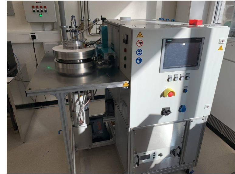
iplas CYRANNUS Microwave Plasma CVD (MPCVD) system for Diamond Growth
